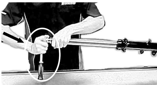
7. Remove the original spring and shims.
