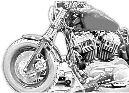
2. Remove the wheel and all the devices connected to the fork following the instructions in the user's manual of the original vehicle.
